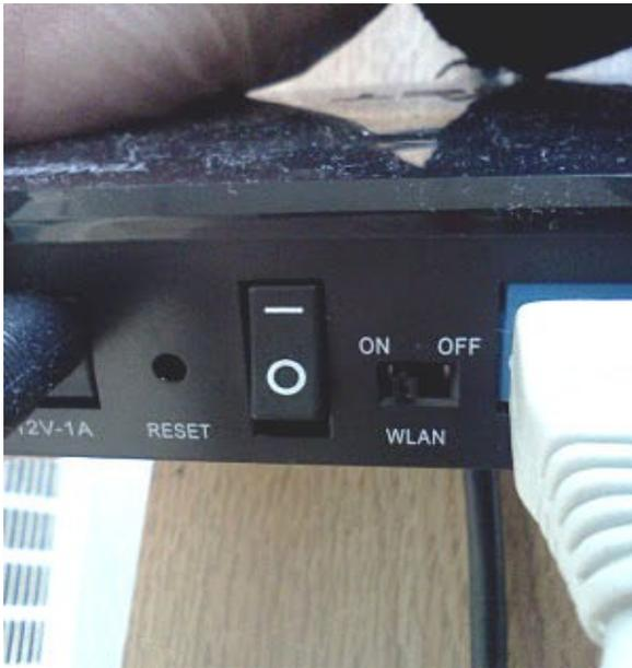
Stick a bent paperclip or a pin in the hole and hold it for 15 to 30 seconds. The lights will go off for a moment and then come back on. It usually takes about 30 seconds for a reboot to complete.
