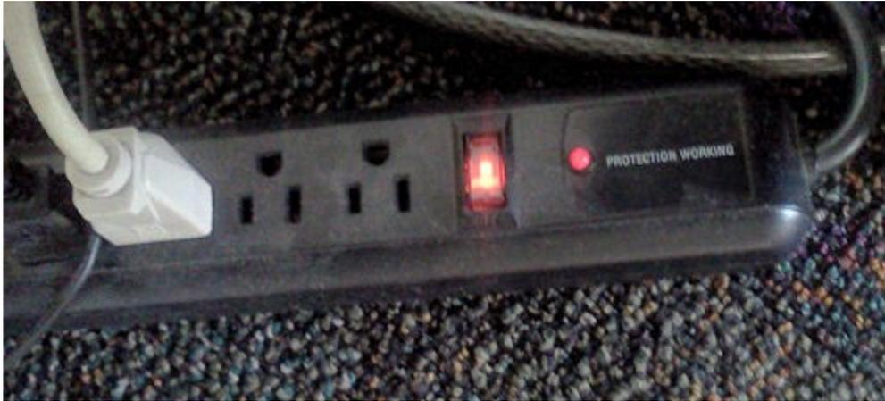
If it isn't lit or you can't tell (the light isn't very bright on some), flip the switch to turn it on. The switch is what is lit up (or should be) so you can't miss it.
