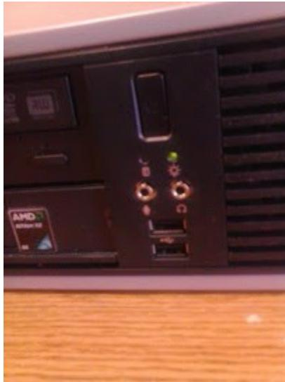
Below the power button in this picture are the headphone and microphone jacks (the two round things), and the USB ports. (Those are the flat, rectangular openings near the bottom.)
